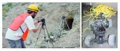
Infrared cameras, enhanced with supplemental infrared lighting, at the mine portal or even mounted on remote-control cars can provide a record of bats using a mine.
